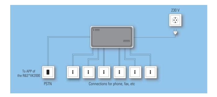
For the optional telephone-operated service within the R&S®XK 2000 family, the radio must be equipped with the internal ALE, APP and EMC filter ALE/APP options.
